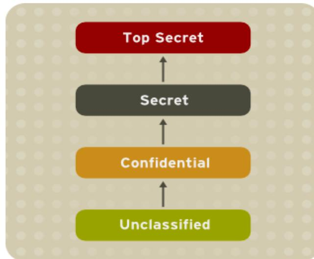
Figure 3.5 Multilevel Security (MLS). (Illustrated by Red Hat (R) Inc. (n. d.))
