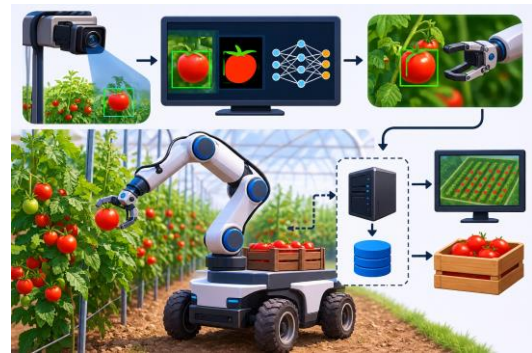
FIGURE 13: Integrated robotic harvesting system architecture using computer vision
