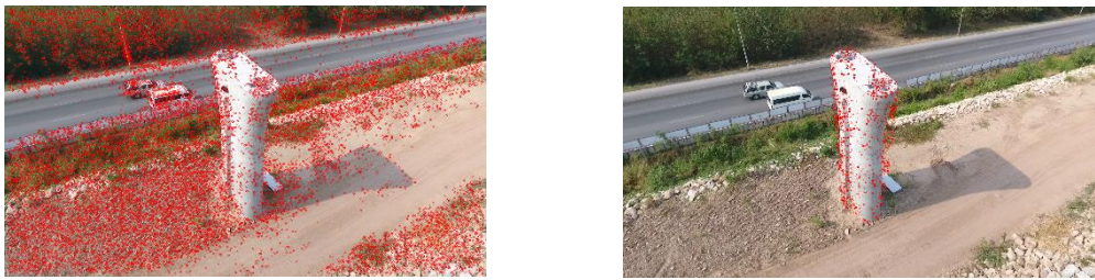
a) All features inside the original image b) Features inside the pier from the proposed system Fig. 8: Comparison between images of all SURF features and SURF features inside the pier (red dots)
