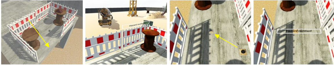
Fig. 7: Unresolved and solved leading edge and floor opening hazards (left and right images, respectively)
