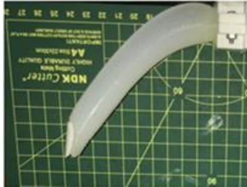
Figure 17. Experimental measurement of soft finger's deformation under pressurization
