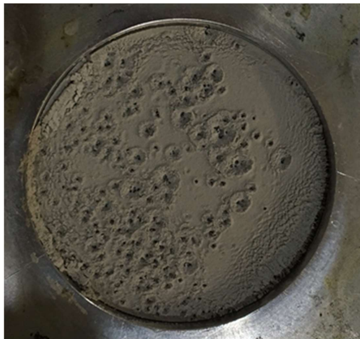
Figure 7 Evidence of scope for ‘pin-holing’ and the presence of pathways clear of build-up (image from a previous study with a different filter media, but identical test conditions).
