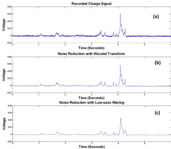
**Fig. 4.** Recorded charge signal and minimising the noise level (a) Recorded charge signal, (b) Noise reduction with the help of wavelet transform and (c) Noise reduction with the low pass filtering.
