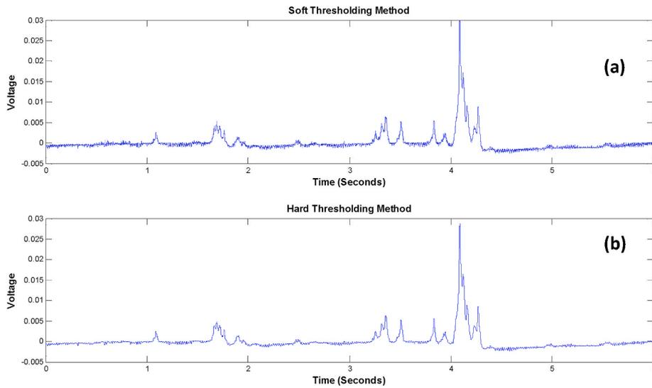
**Fig. 3.** Implication on selection of thresholding type (a) Thresholding of wavelet coefficients with the help of hard thresholding method, (b) Thresholding of wavelet coefficients with the help of soft thresholding method.
