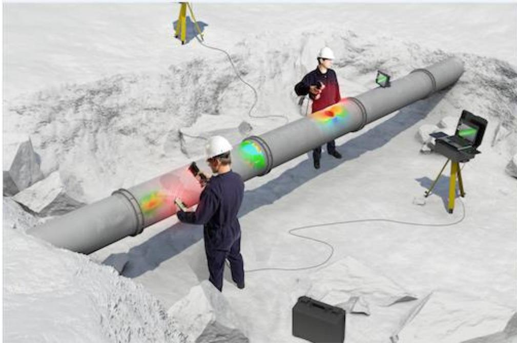
Figure 1.2 Direct Assessment of the pipeline condition in the field (NACE International, 2010).
