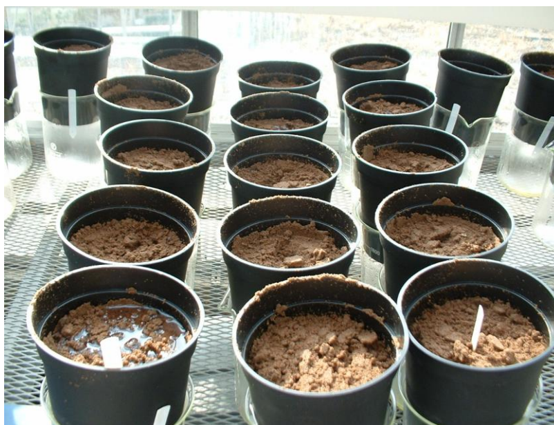
Fig.3.21: Photograph showing water staying on top of the HC-contaminated soil matrix, before quickly running through the holes at the bottom of the pot
