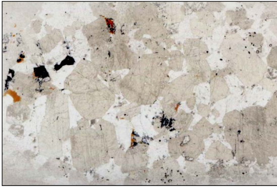
Fig. 5-28. Photomicrograph of Platreef gabbronorite (plane polarised light), consisting of euhedral to subhedral cumulus orthopyroxene and clinopyroxene in intercumulus plagioclase. Minor phases are red-brown phlogopite and opaques. Specimen N1-14. Field of view ~3 cm wide.
