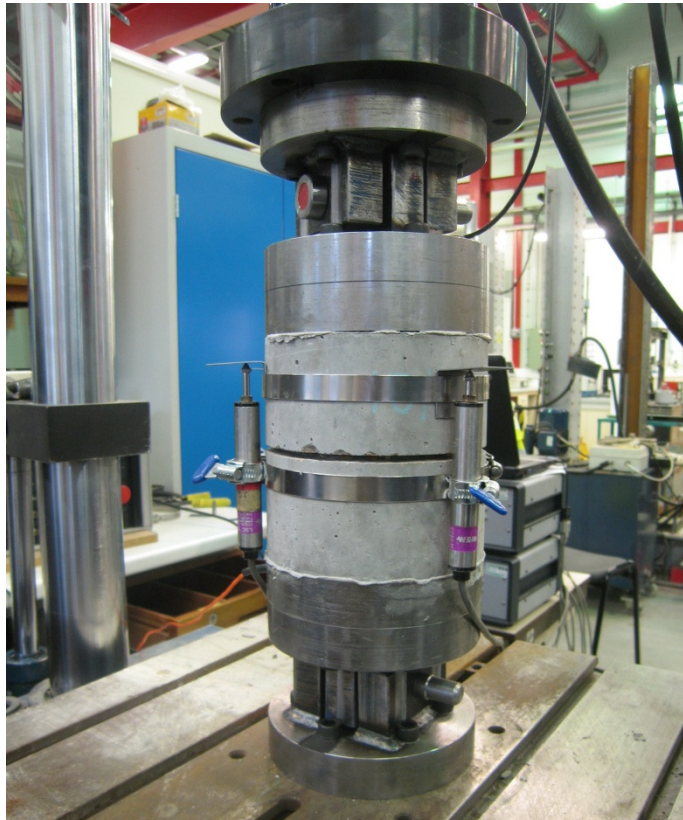
Figure 5-8 Setup of direct tensile test
