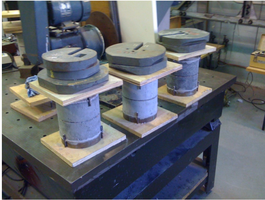
Figure 5-7 Applying small loads on the glued concrete specimen.
