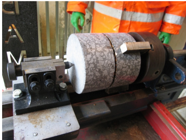
Figure 5-6 Work platform for notching the specimen
