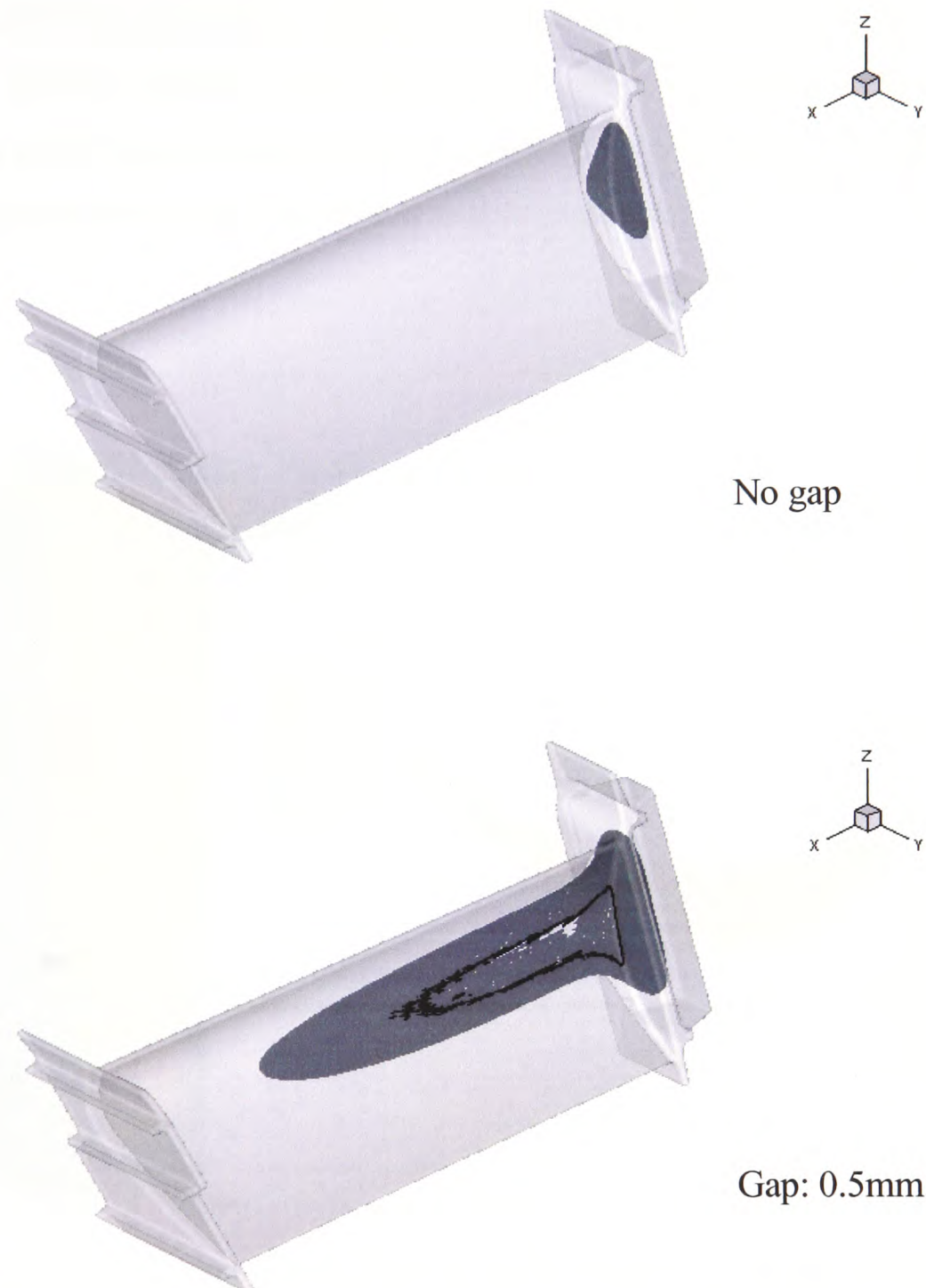
Figure 7.9: Comparisons of the liquid fraction iso-surface ‘LFN=0.35’ of the blade between having a gap and no gap at 130s.
