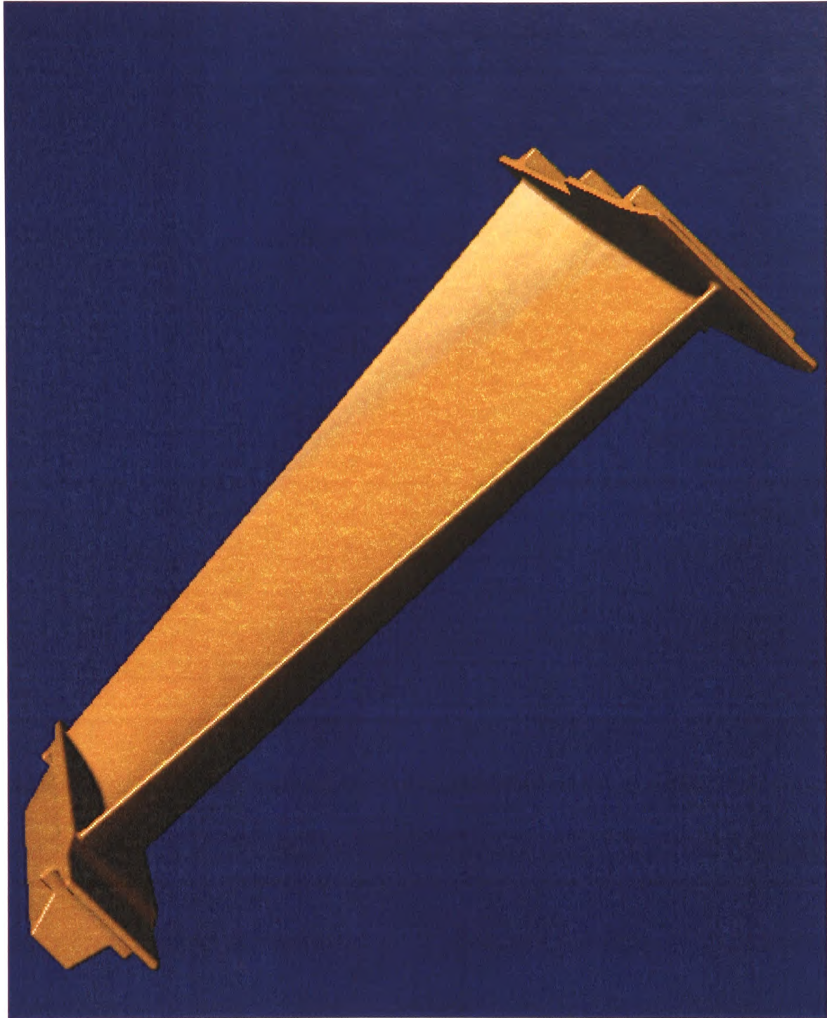
Figure 6.10: Real shape of 400mm long turbine blade.
