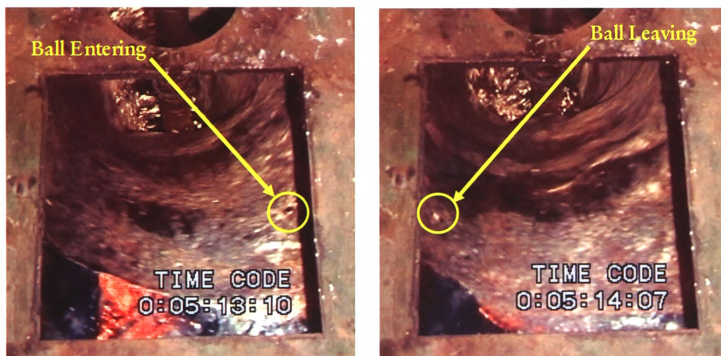
Figure 4.25: Monitoring of Floating Steel Ball Entering and Leaving the Frame
