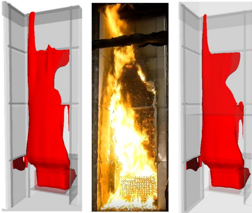
Fig. S13. Observed (middle) and predicted fire plumes at the time to fail in the simulations using the Mesh 3 (left) and Mesh 4 (right) meshes respectively for GCLG test 7.
