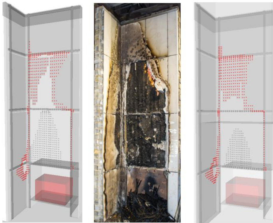
Fig. S14. Observed (middle) and predicted burning locations from the simulations for Mesh 3 (left) and Mesh 4 (right) respectively for DCLG test 7.
