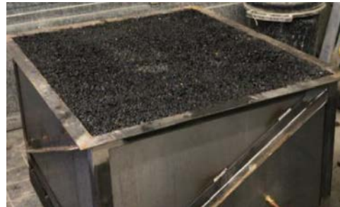
Figure 4. Experimental Rig for Low-Carbon-Porous Asphalt Pavement (LC-PAP) Constructed and Tested at the University of Greenwich, Medway Campus, England, UK (Period of Analysis 2016-2018)
