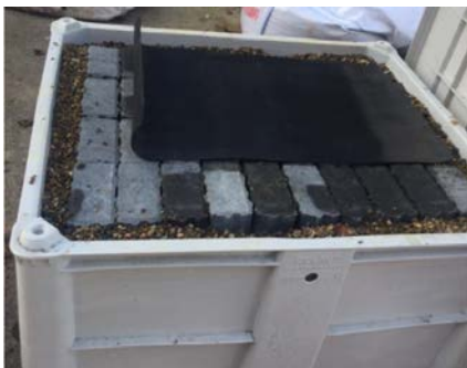
Figure 2. Experimental Rig for Interlocking Permeable Pavement Block System Constructed and Tested at the University of Greenwich, Medway Campus, England, UK (Period of Analysis 2016-2018)
