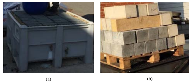
Figure 5. (a) Axial Load Testing for Interlocking Concrete Block Permeable Pavements and (b) Axial Load Testing for Low-Carbon Porous Asphalt Systems at the University of Greenwich, Medway Campus, England, UK (Period of Analysis 2016-2018).
