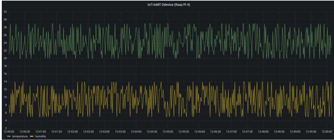
Fig. 3. Randomly generated temperature and humidity values from IoT/IoMT device visualized in Grafana.
