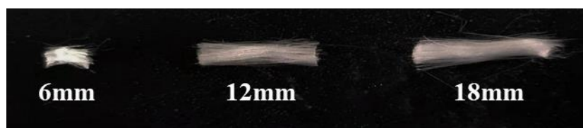
Fig. 2. Photograph of PE fibres with different lengths.
