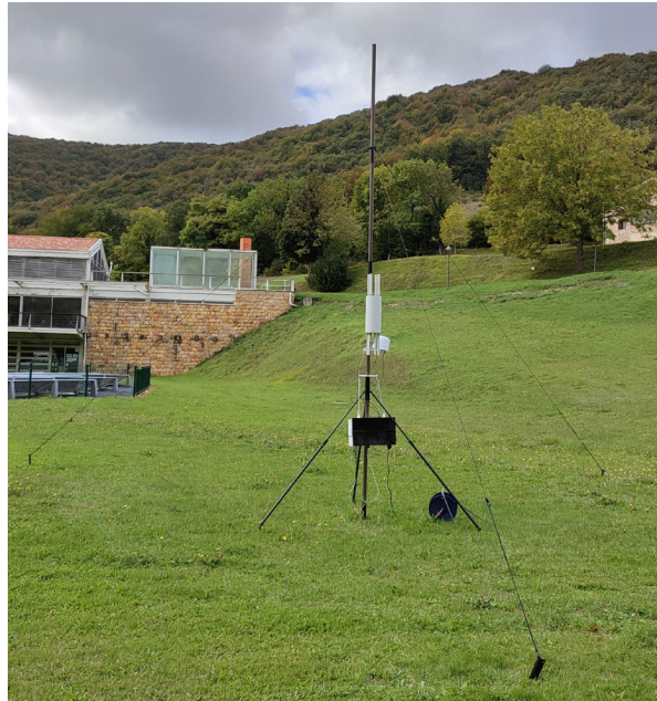
Figure 2. The field communication solution deployed during a Small Scale Field Test. The WiFi 6 access point, with the 4G antenna and the central node can be seen attached to a portable antenna mast.
