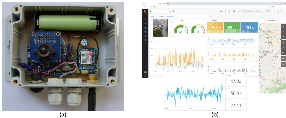
Figure 2. (a) An overview of the electronics and hardware design; (b) User visualization frontend.
