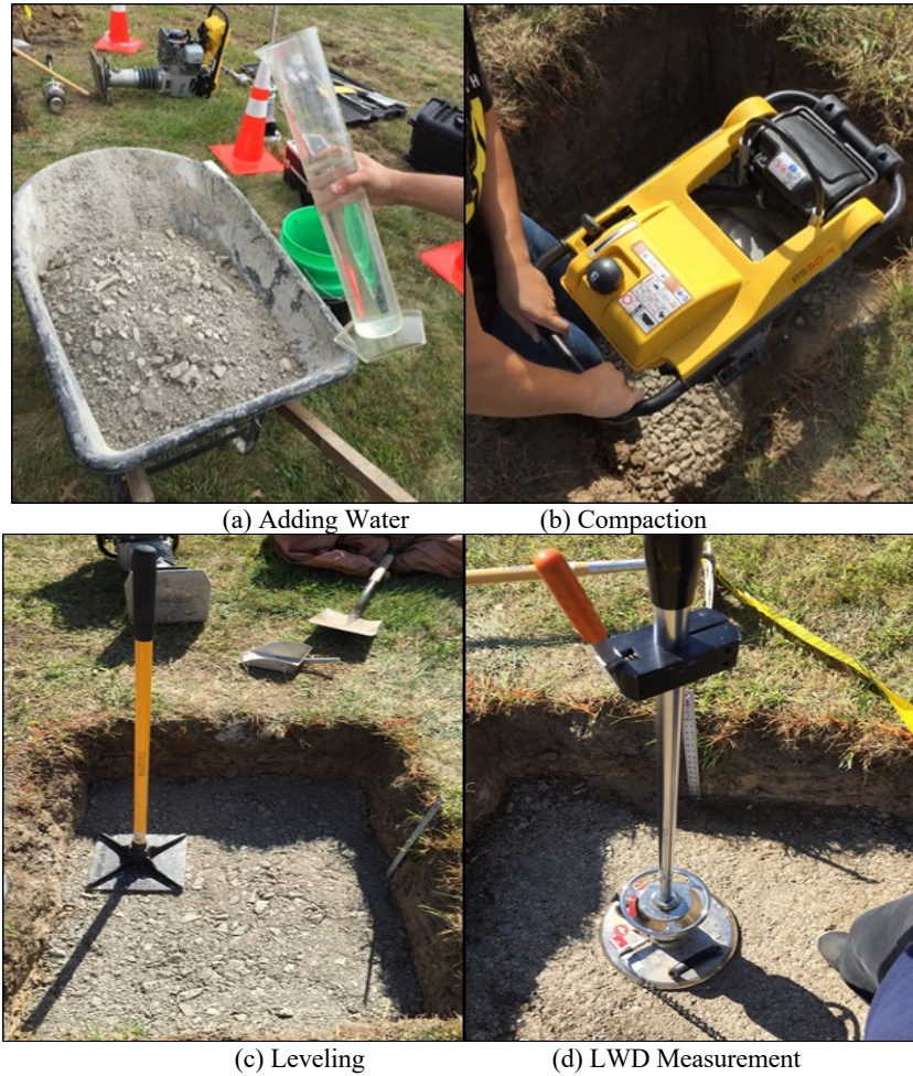
Fig. 8. Test Pit Experiment Process
