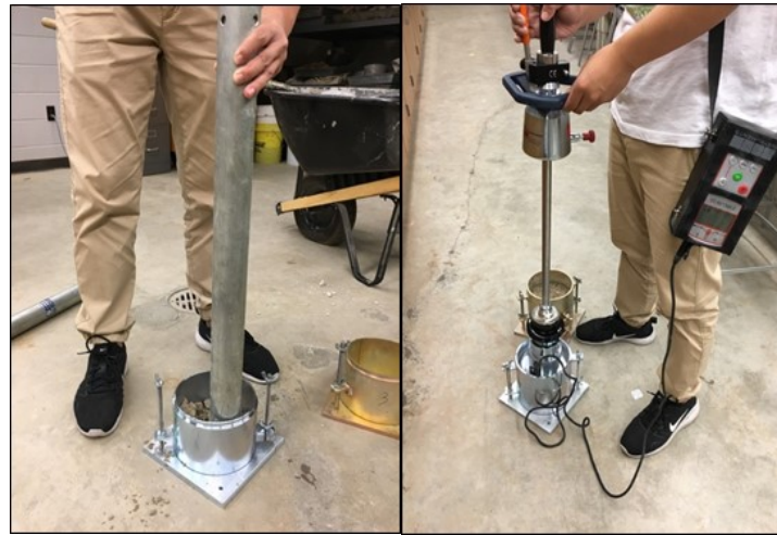
(a) Proctor Compaction (b) LWD Test in Mold
