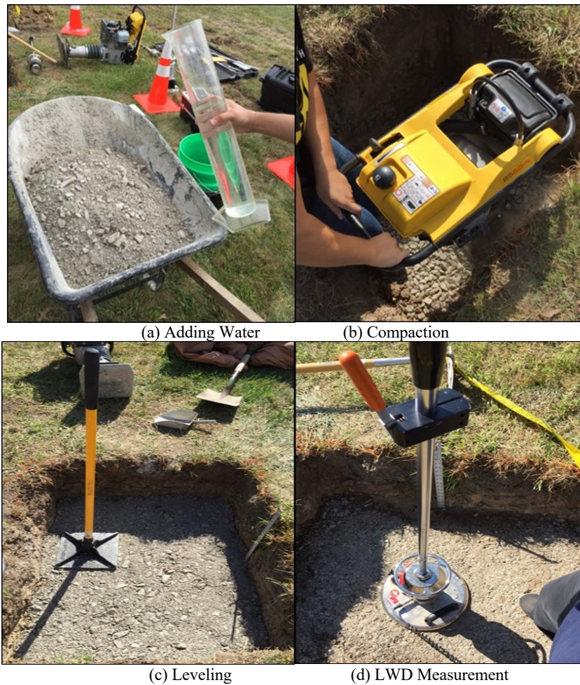
Fig. 8. Test Pit Experiment Process
