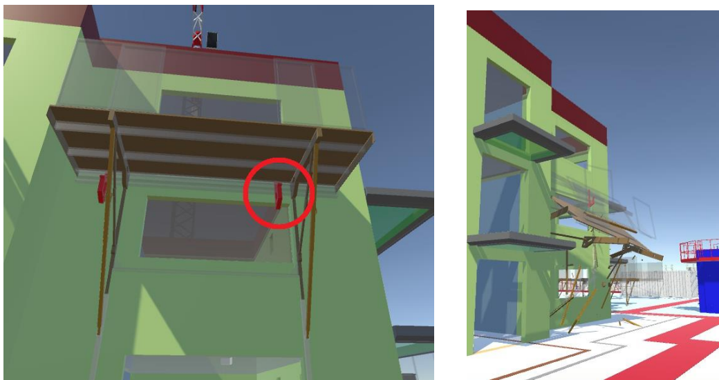
Figure 4: Example of misplacement of fixings of PTE platform in the virtual environment. On the left, one fixing is misplaced (circled in red) and placed above an opening. On the right, this is what the trainee will see if he walks away from the PTE platform if he does not signal the misplacement of the fixing (This corresponds to the bottom left state in Figure 3).
