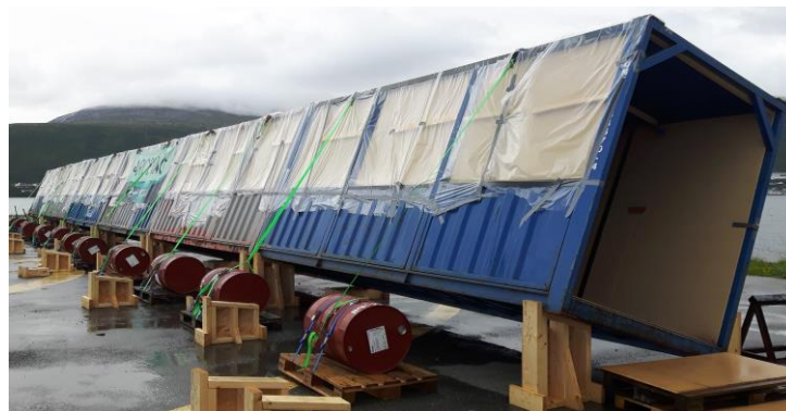
166 Fig. 1: The Tromsø test facility heeled at 20° 167
