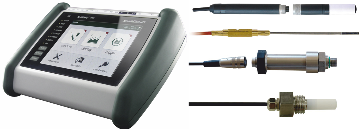
Figure 3 Datalogger plus sensors programmed and installed at CIAT's pneumatic dryer
