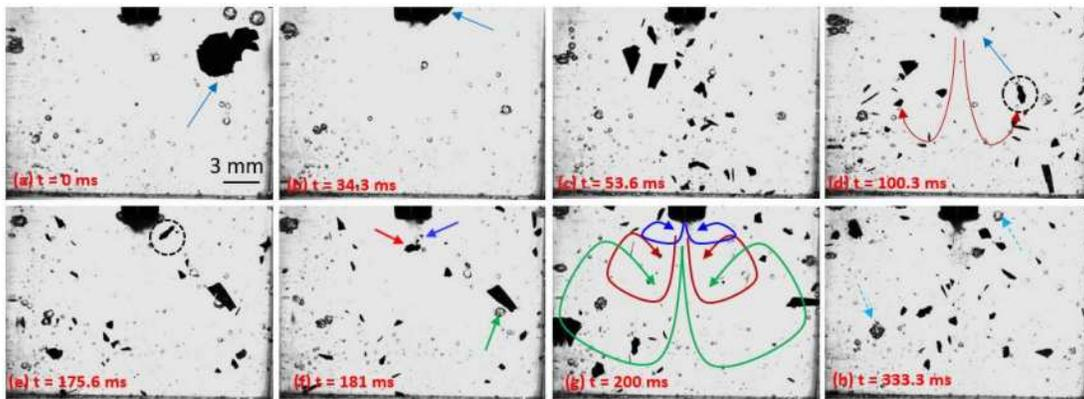
**Figure 2.** Series of in-situ high-speed images (3000 fps) of ultrasonically induced free-floating crystal breakdown.
