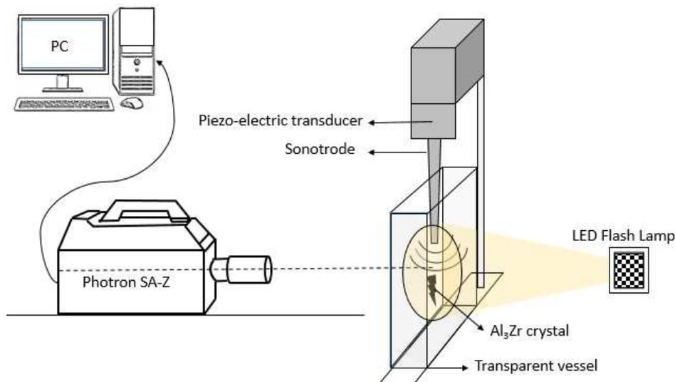
**Figure 1.** Schematic representation of an in-situ high-speed imaging experimental setup.
