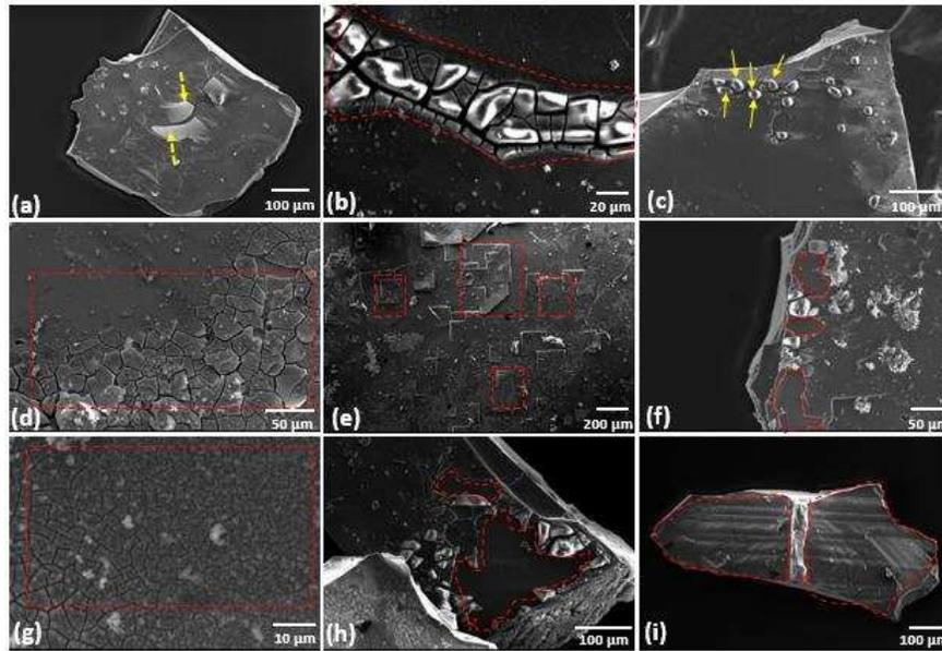
**Figure 3.** SEM images of fragmented crystal after exposure to ultrasonic cavitation for 3 s (a,b,c), 6 s (d,e,f), and 9 s (g,h,i).
