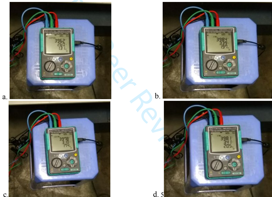
Figure 4. The power consumption at various machining conditions: (a) Experiment no. 1 (Replication-2), (b) Experiment no. 2 (Replication-2), (c) Experiment no. 9 (Replication-3), (d) Experiment no. 13 (Replication-3)
