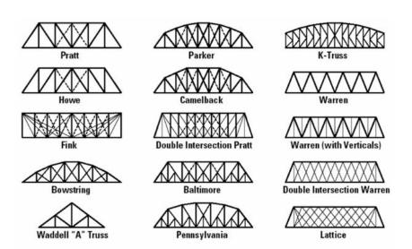
load from a single point to a much wider area. Like the lolly sticks available, historic truss bridges were first made from **wood**. This activity will allow you to experiment with the composition of the truss, discovering which patterns create the most rigid structure.
