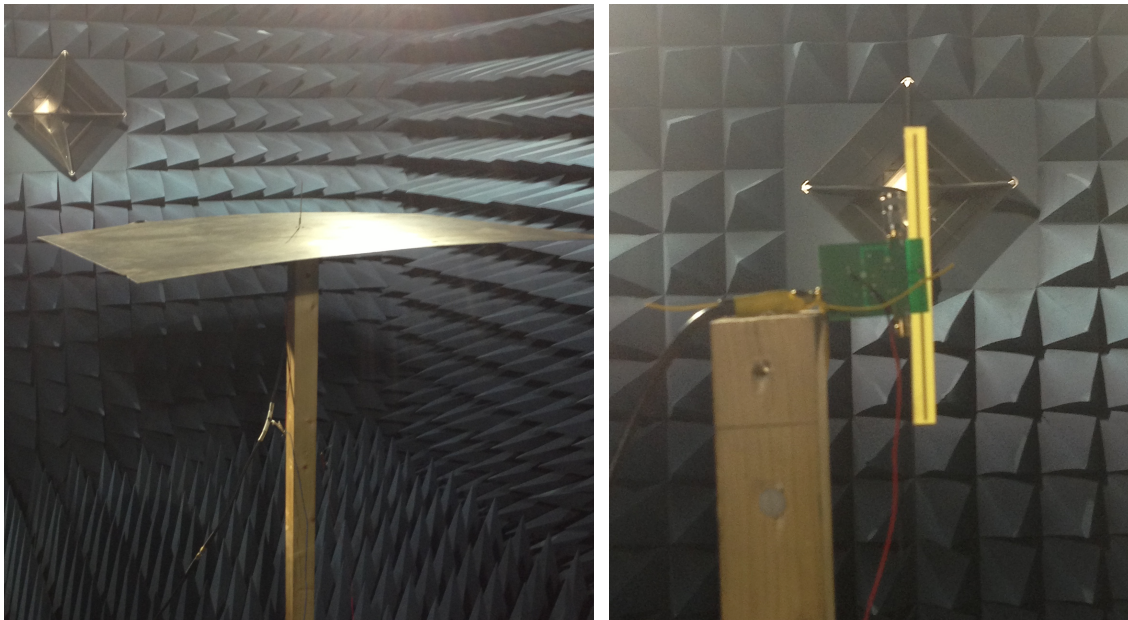
Figure 6.12: Measurement setup of conventionally fed monopole antenna (left) and differentially fed dipole antenna (right)
