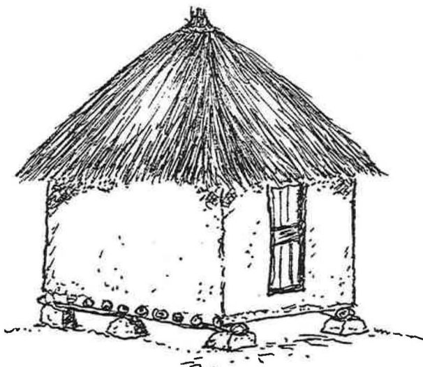
Figure 4. Examples of mud block/brick silos
