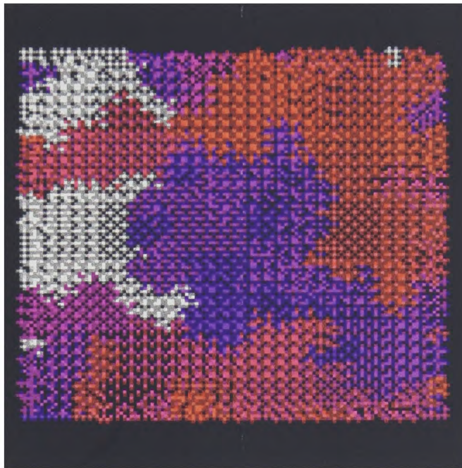
Figure 2.17: Microstructure of solidification, 90^\circ contact angle, 6.5 \text{ K/s} cooling rate and the Ito stochastic dynamics used.
