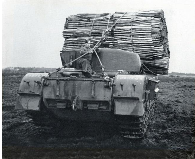
Figure 6.1 Tank with paling for creating trackways (taken from House, 1953)
