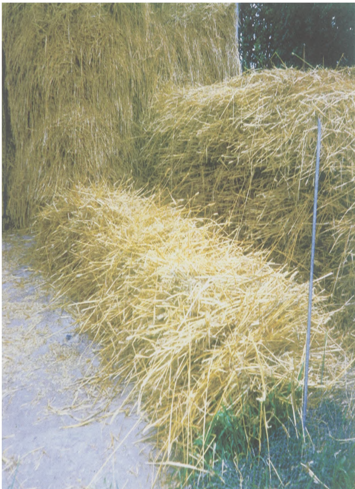
Illustration 21 - A layer of straw, known as a yealm, after it has been drawn from the bed
