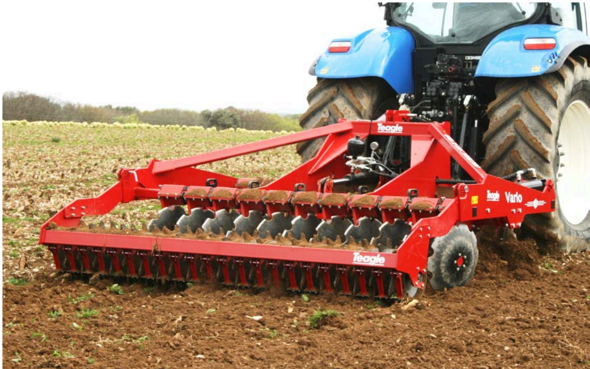
Figure 4.12 Conservation Tillage Using Discs and Tines
